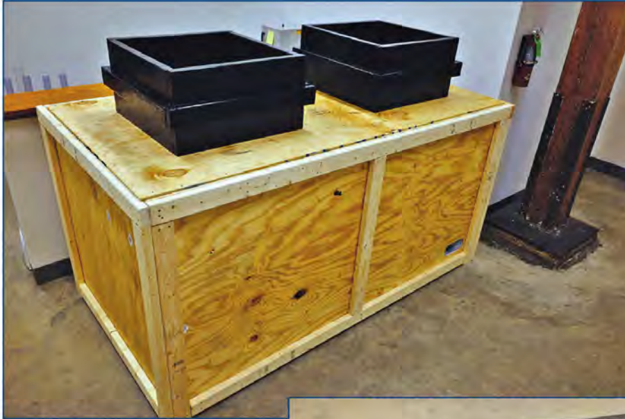
Figure 4 – Test chamber with two panels installed on top.
