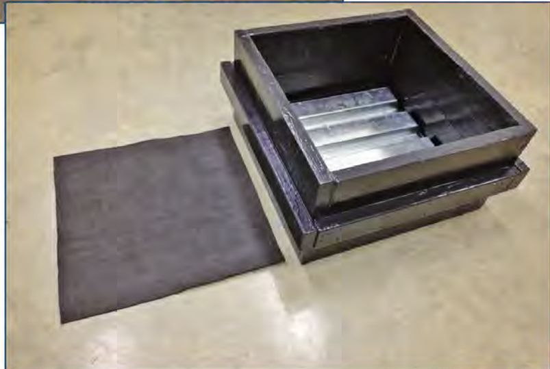
Figure 5 – Non-woven polyester fabric and test panel. The panel box is fully coated in a vapor-impermeable paint.
